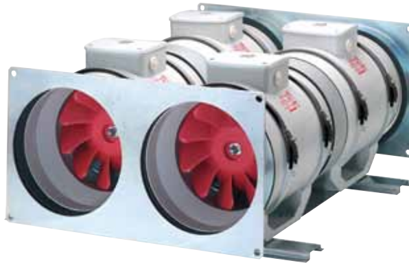
IN SERIES + PARALLEL FOR RECTANGULAR DUCTS (DOUBLES THE PRESSURE AND THE AIR FLOW)
